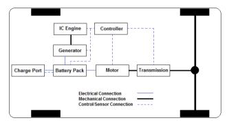
Figure 1: Plug-in series powertrain
