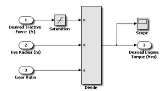
Figure 5: Engine torque model
