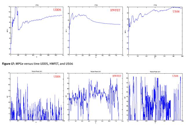
Figure 18: Tractive power (in kWh) versus time for UDDS, HWFET, and US06
