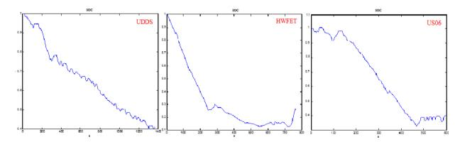
Figure 21: State of charge (SOC) for UDDS, HWFET, and US06
