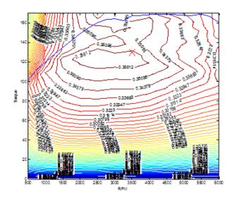
Figure 22: Torque (Nm)-speed (rpm) curve of ICE
